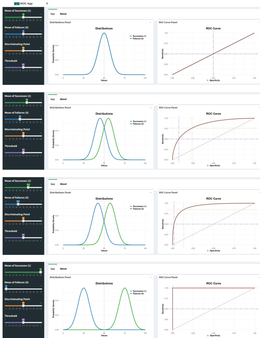
Figure 4 - Area Under the Curve (AUC). The AUC increases from top to bottom as the separation between the distributions increases. This is attained by moving the population slider buttons apart from each other on the control panel.
